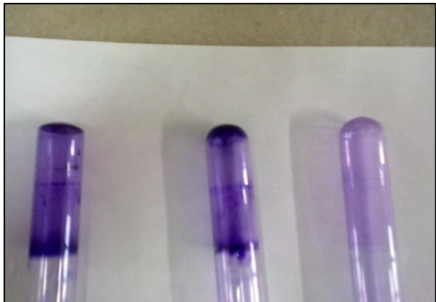
Fig. 2: Tube method showing biofilm formation indicated by staining with crystal violet (first 2 tubes)
